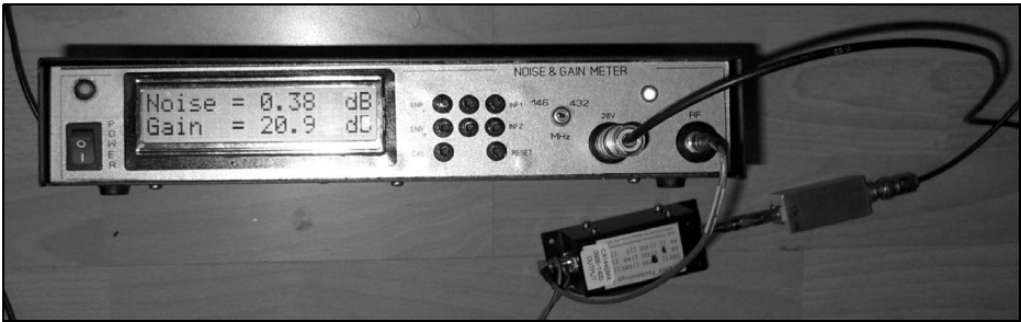
Fig 4: Photograph of the completed Digital Gain and Noise Meter (DGNM).
