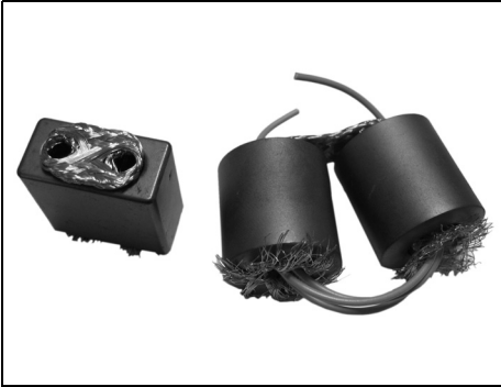
Fig 4: Completed RF power transformers.
