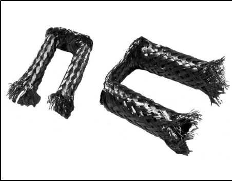
Fig 3: Forming the primary from coax cable shield.
